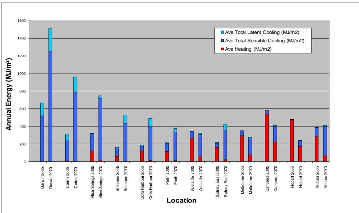
Figure 1: Differences in thermal conditioning energy, 2005 vs 2070 after BRANZ 2007
