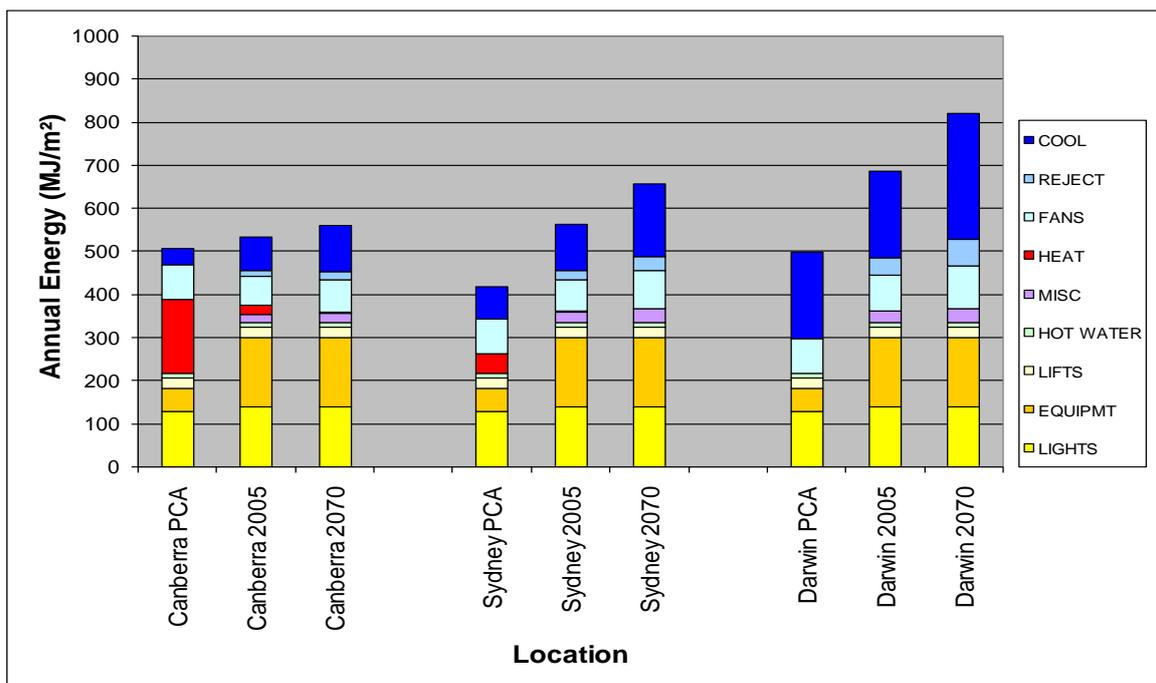
Figure 2: Simulated end-use energy consumption of 10 storey office block after BRANZ 2007
