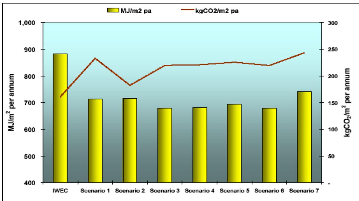
Figure 3: Hospital energy consumption and greenhouse gas emissions based on predicted weather files for Melbourne (after BRANZ 2007)
