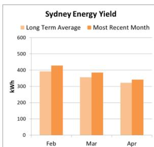
**Sydney** also had cooler and sunnier than average weather in April. The mean maximum and average were lower by 3.6°C and 1.5°C. Only the minimum was higher by 0.5°C. The PV energy yield was 5.4% higher. All 4 facing zones of the 10-storey office had cooling consumptions less than the average. The South-facing zone had over 29% less cooling due to the cooler air temperature. The North zone also consumed less cooling energy but by a lesser amount of 17% due to the sunnier weather.
