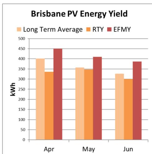
When comparing our EFMY 2050 simulation results with the results for June, it is projected that the two office models would have around 36-45% higher cooling consumption, and the supermarket would have about 28% higher cooling consumption than for the June just gone. The solar PV energy output for June when compared with the EFMY 2050 energy output showed 7.3% lower energy output projected in 2050.
